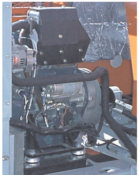
It is a very suitable mount for engines where it is not physically possible to install the antivibration mounts at the same height as the crankshaft.
